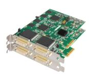
The Radium-I3 Hybrid HD/SD Input Capture Card deliver extreme performance to the Radium Videowall Systems with its 650MB/s transfer bandwidth, capturing 1 High Definition Video Sources and up to 4 Standard Definition Video Sources.
